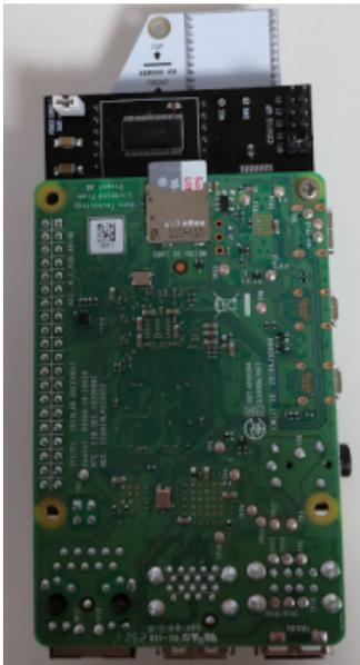
It is mounted on the MPU socket. Since the upper end of the socket is visible, it is possible to visually align the pins.
